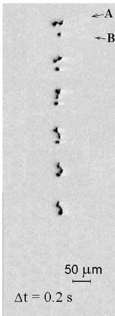
Fig. 16. Sequence of frames illustrating the mutual approach of the agglomerates “A” and “B” (Fig. 14) when the field was switched off. The time interval between the frames is \Delta t = 0.02 s. Time increases from top to bottom.
