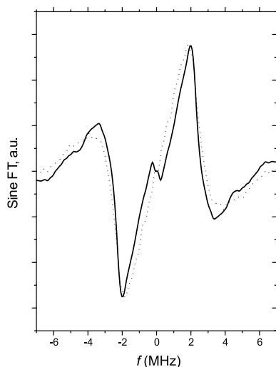
Fig. 2. Fourier transform of ESEEMs given in Fig. 1c for 13 K (solid line) and for 20 K (dotted line). The result is a Pake resonance pattern, which has an antisymmetric lineshape due to spin polarization. The singularities correspond to the perpendicular orientation of the pair, the edges correspond to the parallel orientation. The feature near zero frequency (solid line) is an artifact.
