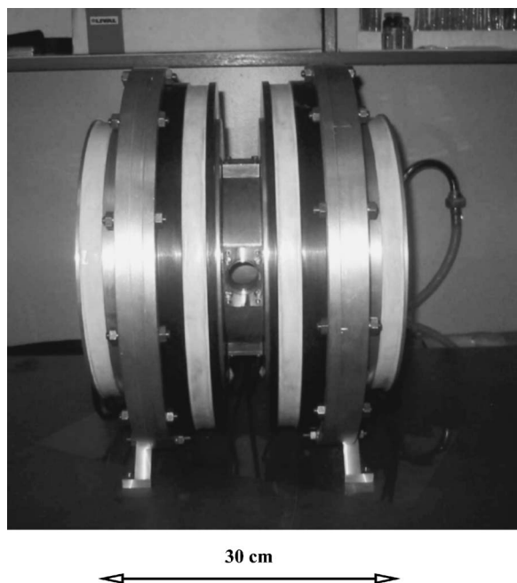
FIG. 12. Photo of the actually built magnetic system, including a 30 cm scale bar.
