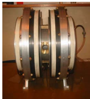
Fig. 2. Left: Schematic cross-section of the magnetic system shown to scale with three pairs of coils in the power system (P), two pairs of coils in the scanning system (S), and the cooling arrangement (C); Right: Photo of the device, outer dimensions slightly under 50 cm.
