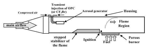
Fig. 1. A scheme of Transient Application, Recirculating Pool Fire (TARPF) Apparatus.
