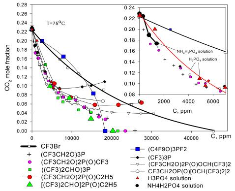
Fig. 3. Cup burner tests: extinguishing concentration of CO<sub>2</sub> as a function of loading of fire suppressants.
