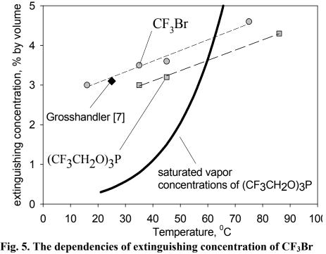
Fig. 5. The dependencies of extinguishing concentration of CF<sub>3</sub>Bi and (CF<sub>3</sub>CH<sub>2</sub>O)<sub>3</sub>P obtained using TARPF apparatus on temperature of extinguishing mixtures (air + fire suppressant).
