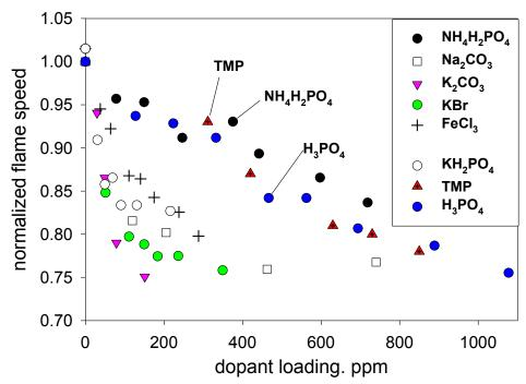
Fig. 2. Normalized speed of a stoichiometric premixed  $C_3H_8/air$  flame as a function of the dopants loading.
