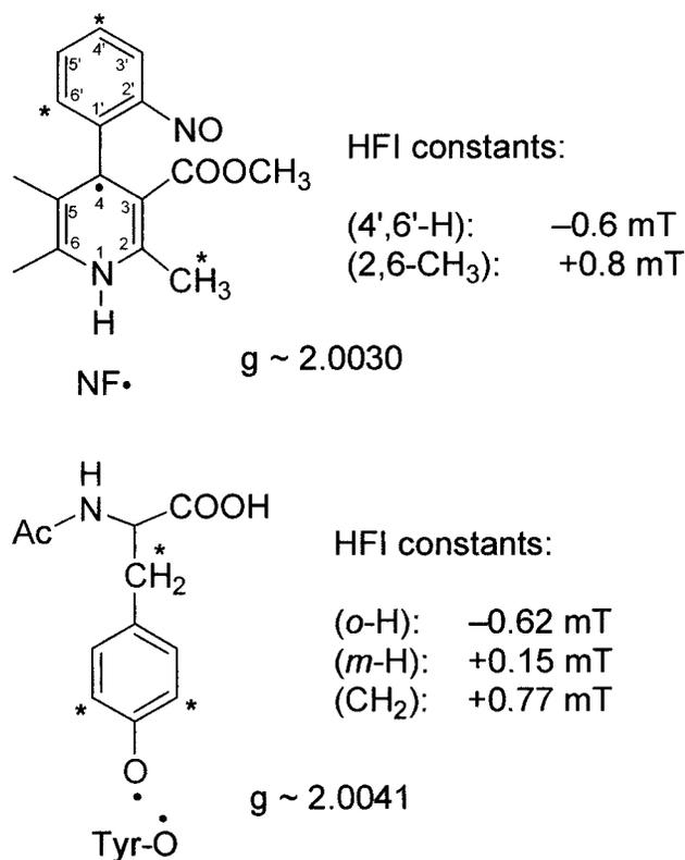
**Scheme 2.** Magnetic resonance parameters (radical  $g$ -factors and HFI constants) of Tyr (15) and NONF (12) neutral radicals (asterisk denotes the protons with the highest HFI constants).
