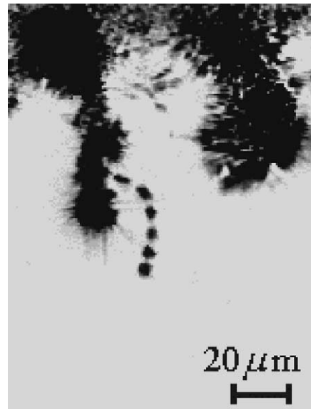
Fig. 15. Video recording illustrating consecutive stages of aggregate-tendril collision. Time interval between stages \Delta t = 0.04 \text{ s} .
