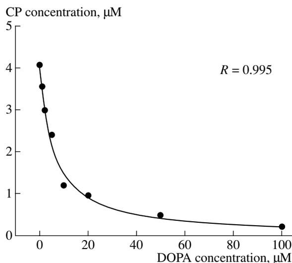
**Fig. 2.** Effect of DOPA on the oxidation of the spin trap CP-H (1 mM) by superoxide. The concentration of CP was determined by the intensity of the EPR spectrum.
