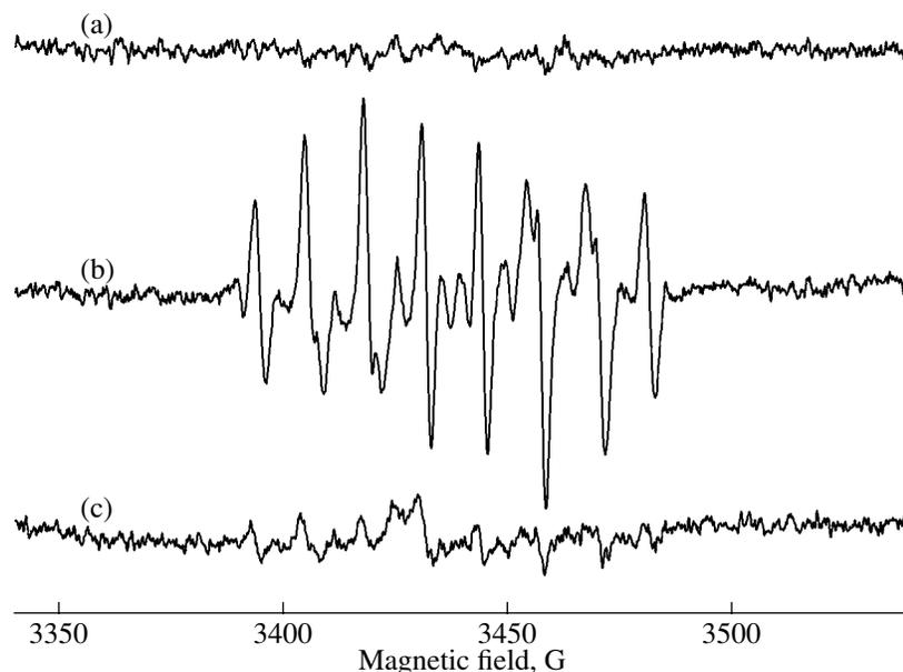
**Fig. 1.** EPR spectra obtained in the presence of the spin trap DEPMPPO (10 mM) during (a) oxidation of DOPA (1 mM) by phenoloxidase (20 U/ml), (b) oxidation of xanthine (0.05 mM) by xanthine oxidase (0.05 U/ml), and (c) oxidation of xanthine (0.05 mM) by xanthine oxidase (0.05 U/ml) in the presence of DOPA (10  $\mu$ M).
