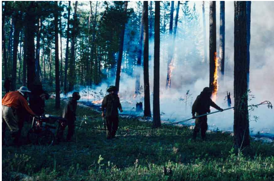
Figure 2. A Russian researcher using a filter probe held over an active portion of a fire to collect aerosols. A pump with a known flow rate collects smoke samples through the probe and deposits them onto filters for later analysis (apparatus on wheels to the left side of the image).
