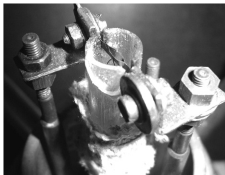
Fig. 2. Photo of a device for polymer degradation study at a HHR by MBMS thermal analysis with time-of-flight mass spectrometer.
