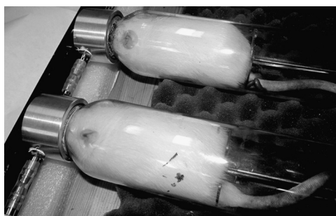
Fig. 7. View of the nose-only exposure chambers connected in series for the inhaled dose measurements.
