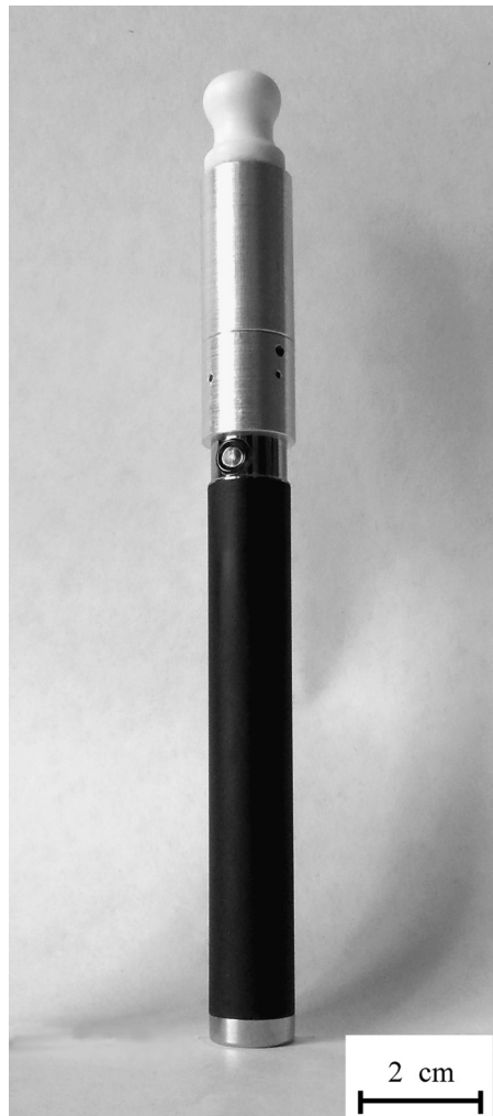
Fig. 3. Portable evaporation–nucleation inhaler intended for humans.
