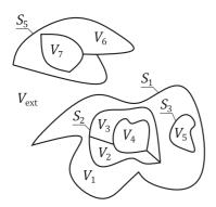
FIG. 5. An example of a multibody multilayered scatterer with piecewise-smooth boundaries and interfaces (having a finite number of edges and vertices). Each  $S_i$  is a closed connected surface, but not necessarily a regular one; it separates at least two domains, one of which may be the external medium.
