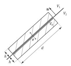
FIG. 3. An exclusion domain for deriving the boundary condition for  $\mathbf{E}(\mathbf{r})$  consisting of two oblate rectangular prisms. The width perpendicular to the image (not shown) also equals *d*. Gaps between the prisms and the locally flat interface are shown solely for convenience. The dashed central line denotes the variation of  $\mathbf{r}$  used to calculate the limit when approaching the interface.
