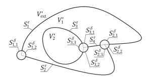
FIG. 7. An example of the exclusion of shape singularities from the interfaces and volume domains. See the main text for an explanation of the symbols; the dashed lines denote the parts of the original irregular surfaces  $S_i$  (cf. Fig. 5) falling inside the neighborhood of singularities. Each  $S_j^r$  is a regular connected surface separating exactly two domains, one of which may be the external medium.
