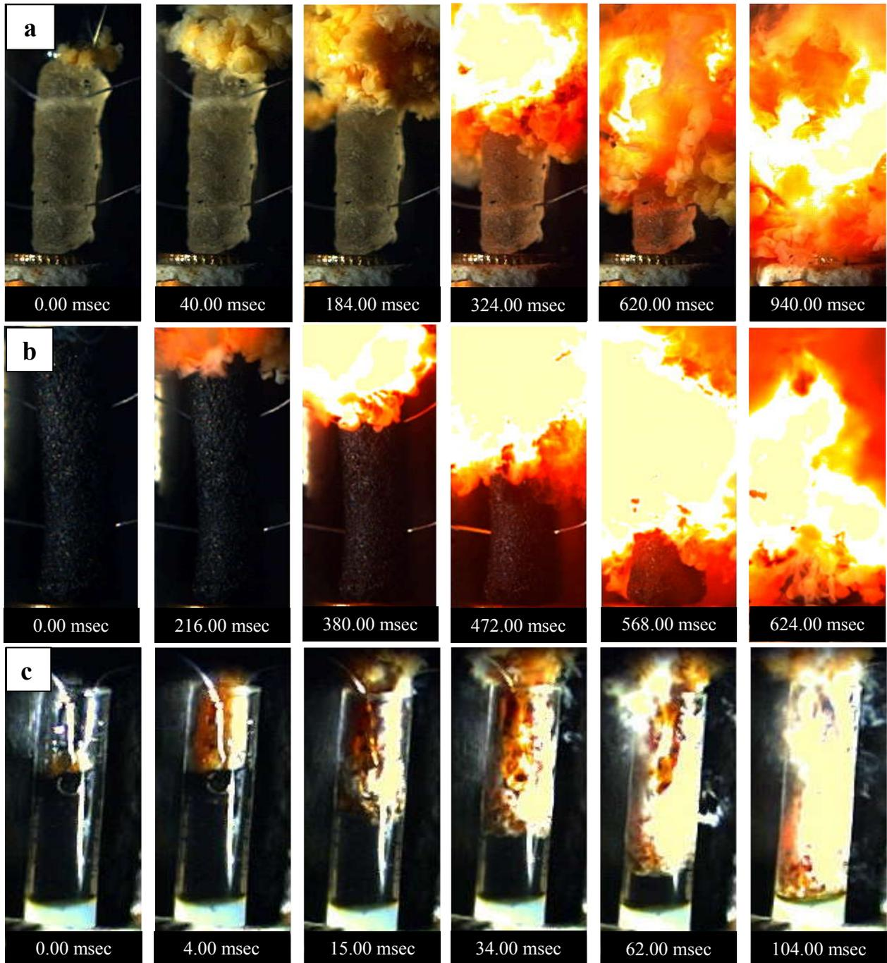
**Fig. 2. Captured images of regression process during combustion of HAN based propellant with various additives.**
