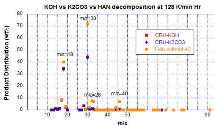
**Fig. 7. Comparison of product ion distribution for KOH and K<sub>2</sub>CO<sub>3</sub> activated carbon and pure HAN without carbon at 128 K/min heating rate**
