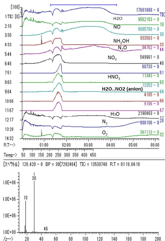
**Fig. 5. EI-MS analysis of total gaseous products of decomposition of HAN with carbonized**
