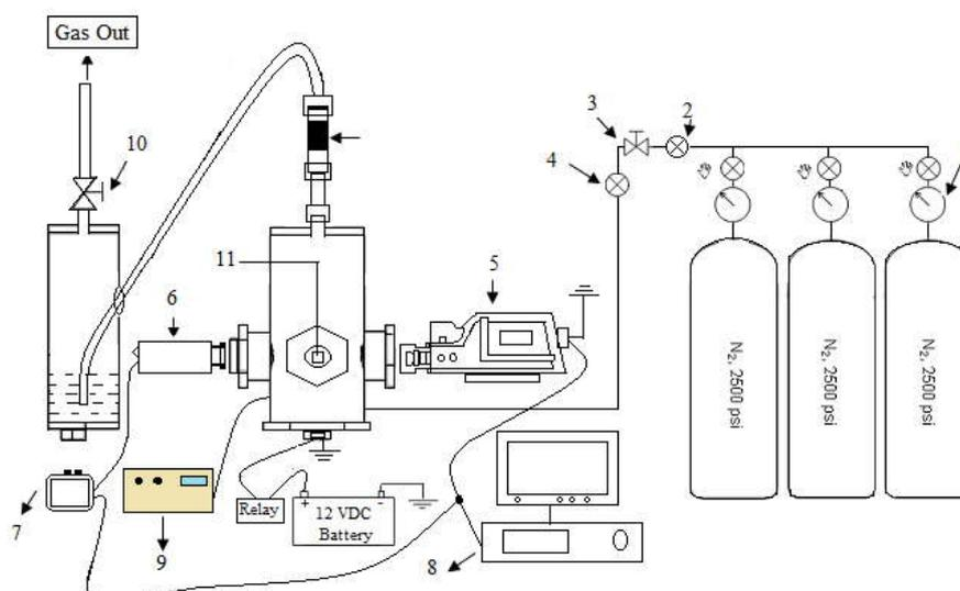
**Fig. 1. Scheme of an enclosed bomb to testing of burning rate**
