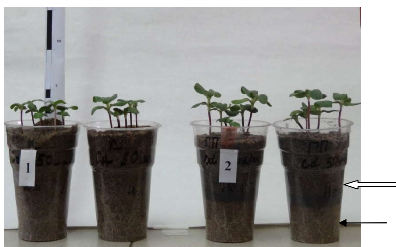
1 - control contains 50 mg/kg of Cd, 2- the experiment the lower layer contains 50 mg/kg of Cd 2+ and a layer of hydrophobic sand. The upper arrow points at a layer of hydrophobic sand. The lower arrow – soil ground with Cd 2+
