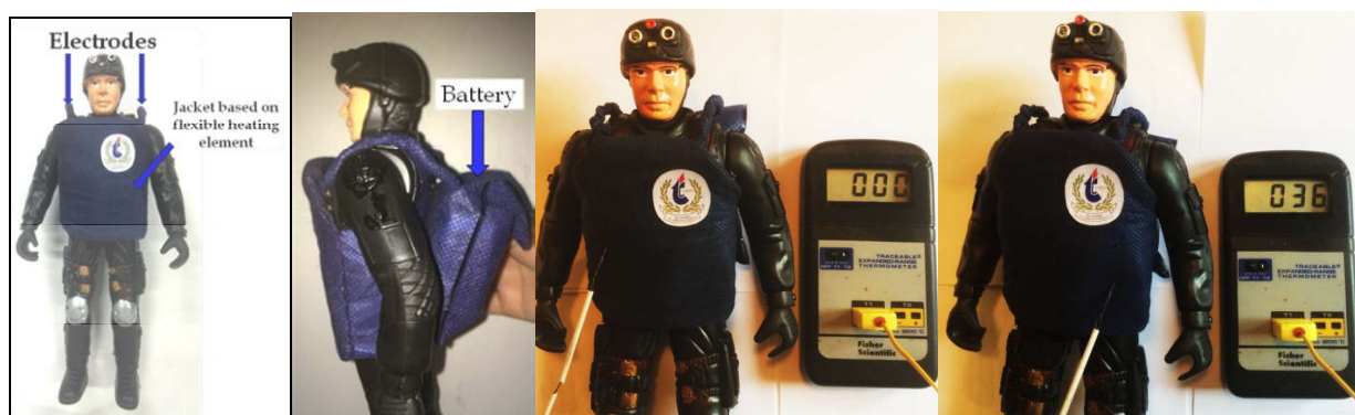
Figure 10 – Photos of soldier model with a jacket based on glass cloth with carbon nanotubes coating and dynamics of jacket temperature changes before the connection and after connection to the power source
