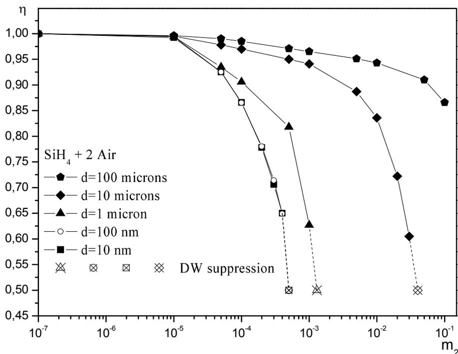
Fig. 1. The dependencies of DW velocity deficit in the stoichiometric silane-air mixture on the inert particles volume concentration.
